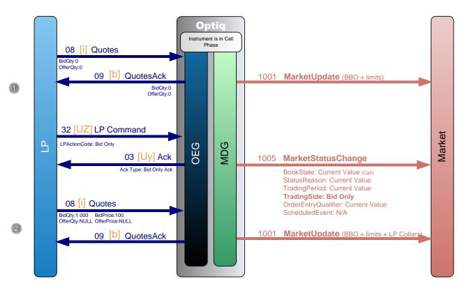
When a Liquidity Provider animating an instrument has no more instruments to sell, he moves to a Bid Only situation by entering the appropriate command. This command can be entered only if the Liquidity Provider has no more Quotes on the Instrument.
