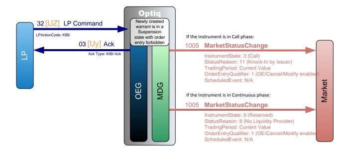
A Liquidity Provider has the ability to unsuspend a newly created warrant instrument by sending a private **LiquidityProviderCommand** (32) (FIX UZ) (Knock-In request). OEG sends back a private **Ack** (03) (FIX Uy) message to confirm the successful receipt and technical processing of the command.
