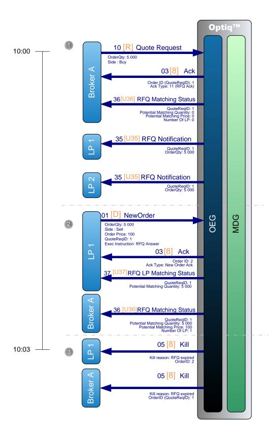
① A Broker sends a private **Quote Request** (10) (FIX R) message to broadcast a new RFQ order with a quantity of 5,000. OEG sends back a private **Ack** (03) (FIX 8) message to confirm the successful receipt and technical processing of the RFQ. This Ack message is an "RFQ Ack", as a consequence the OrderID will contain the QuoteReqID.
