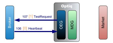
After n second(s) of inactivity on the broker side (i.e. when the OEG has not received any message since n second(s)) the OEG sends a **TestRequest** (107) (FIX 1) message to the broker.
